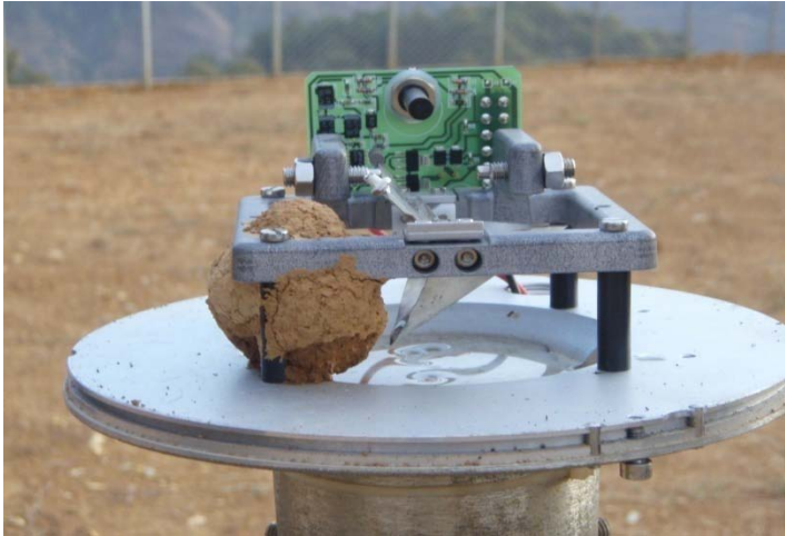
Mud housing by Wasps blocking tip of rain gauge
